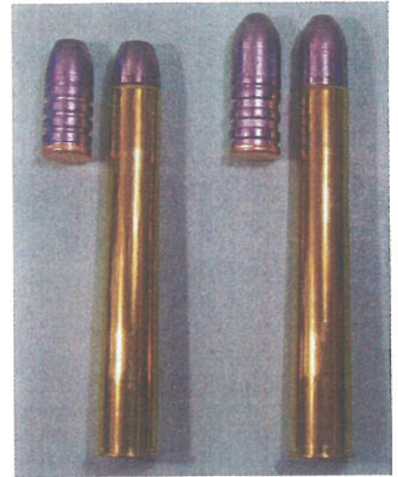
A 420-grain RCBS bullet and loaded cartridge, left, and a 520-grain Mountain Mould bullet and loaded cartridge.
