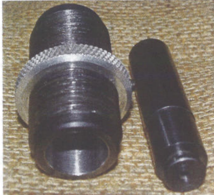
The bullet-sizing die made to size projectiles down to 0.731".
