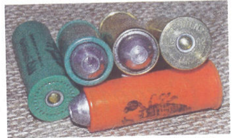
Activ plastic and RMC Lathe-turned brass cases loaded with CBE hollow-point and solid cast lead projectiles.
