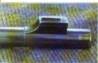
Above, the front sight is an extremely low gold blade dovetailed and screwed to a small base, the latter integral with the barrel. Above right, brazed to the barrel, the rear sight has leaves regulated for 50, 200 and 300 yards.
